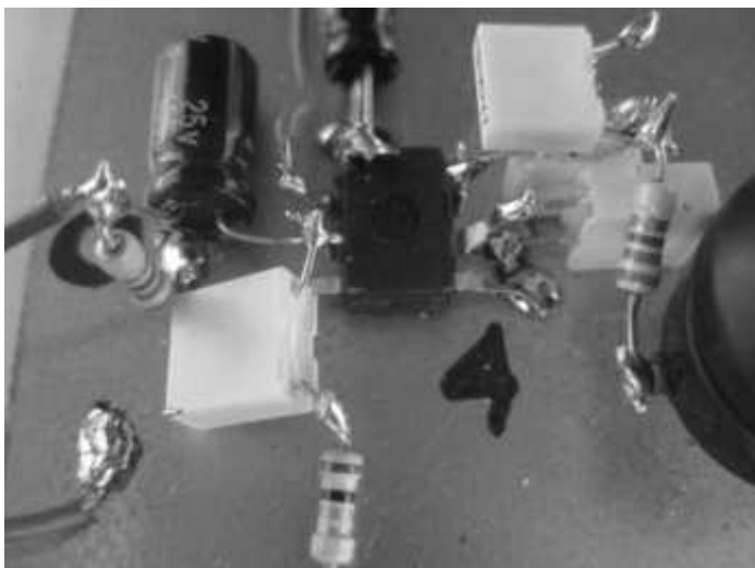
Above – Dead bug technique - Block 1 Left – Output stage IC100 close up
