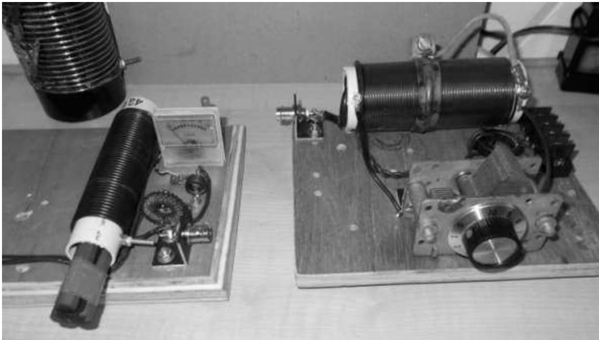
Counterpoise tuner on left and main AMU on right in photo above.
