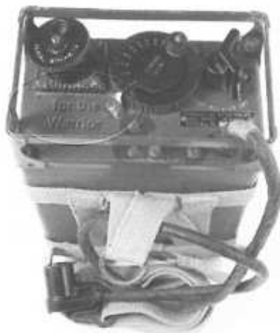
Type D Wavemeter spot frequencies 1.9 - 8.0Mc/s in two ranges. The gaps filled by VFO (centre knob) with 1 MHz pips to 25Mc/s. Worked off 6V cell
