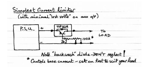
Below the current limit set by the base current (collector current = Hfe x base current), the transistor feeds the circuit as a saturated switch, with only Vce-sat, (0.2v or less) drop.
