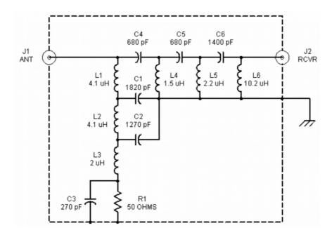
Joe's design features a low pass filter and a high pass filter, which, coupled together, block a full band of frequencies, the A.M. broadcast band. This allows our LF / VLF brethren to operate seamlessly  $VLF \rightarrow LF \rightarrow HF$  without having to exchange filter modules, a great idea if you're into HF and LF operating all at once!
