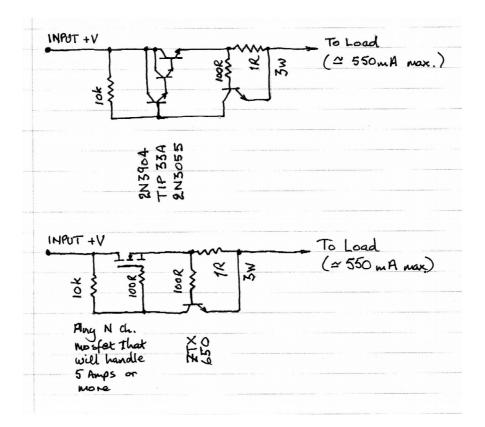
Note: you might need a 'backwash' diode on the Darlington circuit. You can set the maximum current with the 1R sense resistor: R=V/I, and V=V be of the sense transistor (ZTX650). A sense resistor of 0.47 $\Omega$  will give 0.55v/0.47 $\Omega$ , = 1.17 Amps, for instance.
