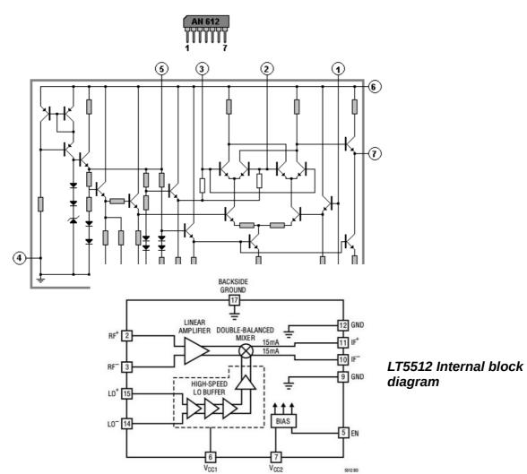
The LT5512 is a similar beast; it has a very high spec. and is a very capable device (but not cheap). Note the enable pin ('EN'). This allows the bias circuits to be switched off for muting and the like.
