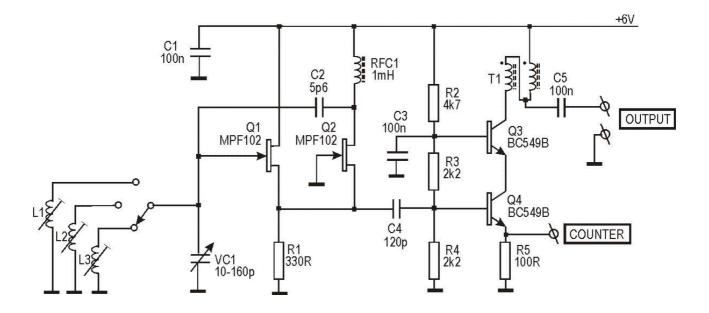
Andrew describes this as a signal generator, but those familiar with low voltage power output stages will recognise transformer T1 as being capable of a good few hundred milliwatts, if not a watt or so, of output. The design is simple, but elegantly sophisticated: much like quality commercial or professional equipment.
