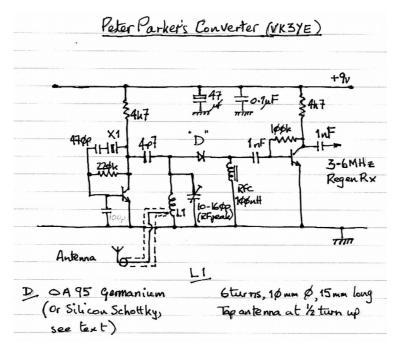
(Note: oscillator transistor base capacitor = 100pF)
