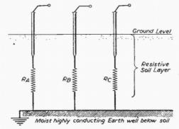
Fig. 1 .--- The arrangement necessary for measuring earth resistance.
