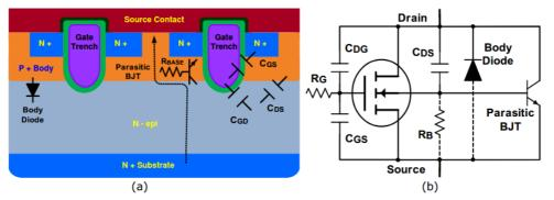
Illustrates clearly the parasitic devices created when constructing the device in silicon. Not perhaps as simple as you expected? And then you wonder why this thing 'hoots' at many MHz with a sniff of feedback and a few pF's and  $\mu$ H's?!
