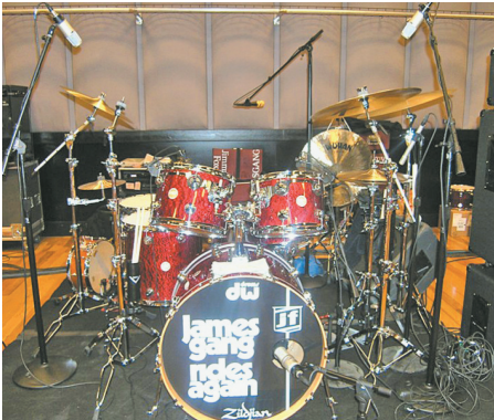
The 100 watt guitar amp is less than 2' from the right PR 30 over the cymbal but yet the incredible rear rejection of the Heil PR 30 that guitar was hardly detected in the overhead channel!
