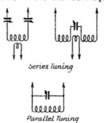
Fig. 2 — Circuits for series and parallel tuning. Separate series condensers may be used in the feeders or a single condenser may be used at the center of the coil to maintain balance.
