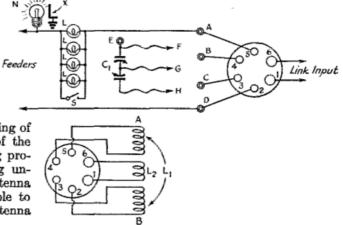
Fig. 1--Circuit diagram of the low-power antenna tuner.
