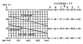
Chart for 14-Mc. band. With end feed, use series tuning for A, C and E; parallel for B, D and F. With center feed, use series tuning for B, D and F; parallel for A, C and E.
