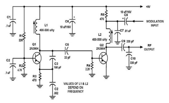
In both circuits the audio input should be sufficient to give 10 - 90% modulation; don't overdrive!!
