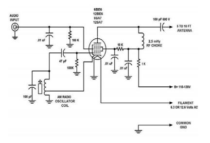
The diagram above shows a Hartley VFO, a crystal can be substituted for "rock solid" stability.
