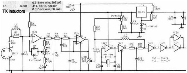
The diagram is part of a D/F Tx/Rx schematic that illustrates how a logic gate can generate Pulse Width A.M.
