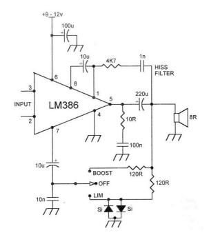
This circuit is so simple, yet delivers so much from a minimum of components. Beautiful! Should the circuit oscillate on "Boost", then increase the 120R "boost" resistor up a tad; try 150R or 180R.
