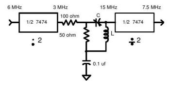
Figure 3 : 6 MHz to 7.5 MHz multiplier
