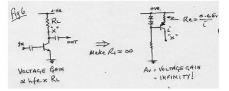
One use - and this one really caught my attention when I first saw it - is the "infinite gain" amplifier shown above in Fig. 6, using one ordinary audio transistor as the amplifier device. The constant current circuit feeds current into the collector (at point "X" above) of the gain stage; gain ~Hfe x RL. If RL approaches infinity ohms, gain = infinity!
