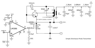
I wonder how many "pirates" tried this circuit (the Michigan Mighty Mite) on A.M. without an RF choke between the LM386 output and Q1 emitter, and to pin 3 of the LM 386? Hah!
