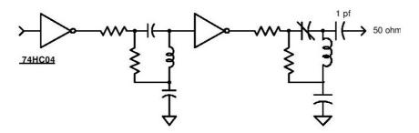
Figure 2: 6 MHz to 30 MHz multiplier with sinewave output.
