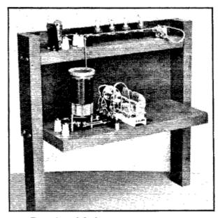
Rear view of the low-power antenna tuner.
