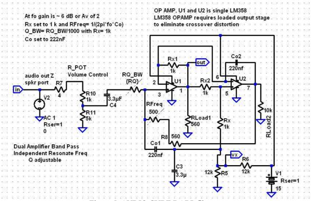
Figure 5: AUDIO CUBE DABP filter structure
