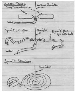
It has always seemed a bit of a oddity to me that we spend any amount of effort in the "radiating" bit of an antenna as it is suspended, cut, trimmed and generally laid out in a tight geometric form: yet the counterpoise, forming the return path to the transmitter, is any old bit of wire strewn about in any manner that will fit. Common savvy surely says the counterpoise should be aligned with the radiating element(s)?
