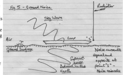
curvature, thus is inducing strong earth currents over a larger area than, say, 30m and higher frequency signals which have a tighter "footprint" as they return to earth from the ionosphere.
