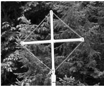
Figure 7 — This photo shows the loop receiving antenna.
