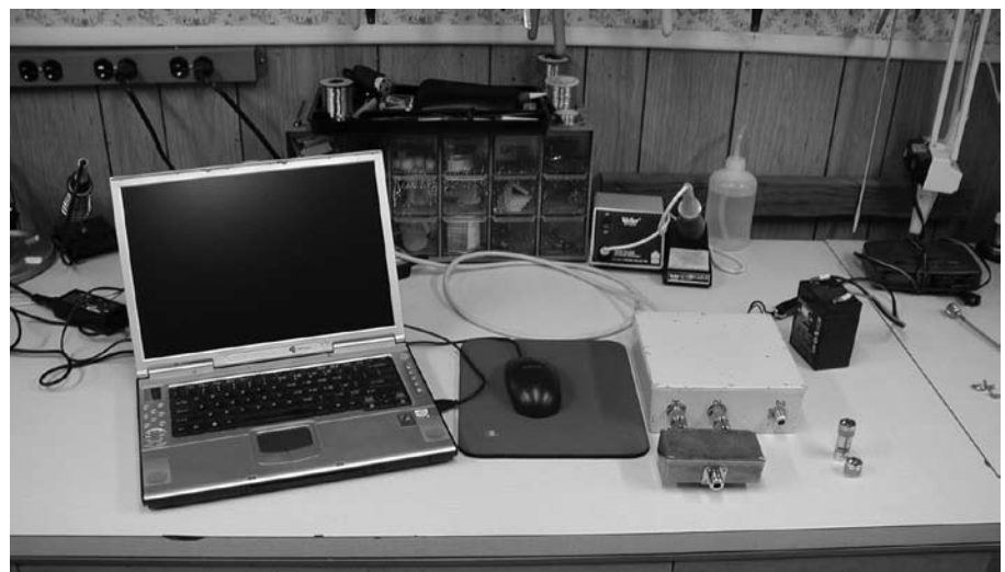
Figure 10 — Here is my test bench, showing the N2PK VNA with the associated laptop computer and HP calibration loads.
