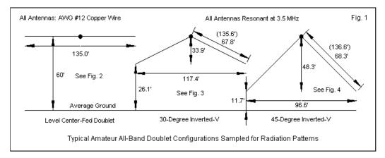
If we start on the right in the figure, we can see why I chose the 60' feedpoint height. The wire ends are between 11' and 12' above ground. Letting inverted-V ends go any lower is an invitation for someone to receive an RF burn, since the wire ends will carry a high voltage when we transmit. Hence, safety dictates that we keep the inverted-V ends at least 10' above ground, and higher, if feasible.
