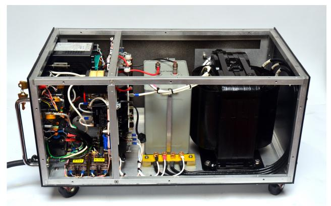
Figure 5: The 67 lb plate transformer, filter capacitor and bleeder resistors mount behind a subpanel that isolates the high voltage components from the control circuitry.
