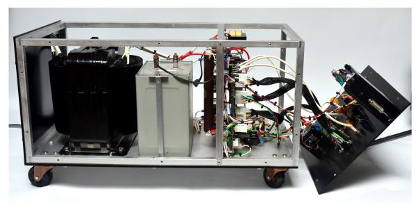
Figure 6: The front panel detaches and tilts forward for servicing and access to the logic and control circuitry.
