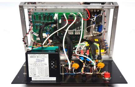
Figure 8: The front side of the subpanel houses the controller printed circuit board, the low voltage transformer, and the step-start circuits.
