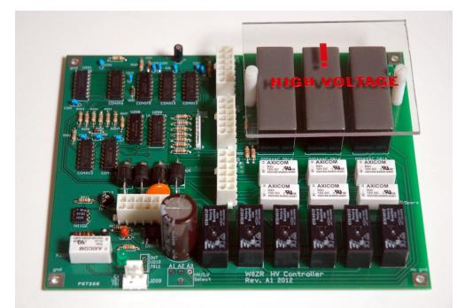
Figure 10: The double-sided printed circuit board houses the logic and control functions, the over-current protection circuit, and the control relays. A plastic shield covers the Gigavac HV relays to keep nearby wires and cables at a safe distance.
