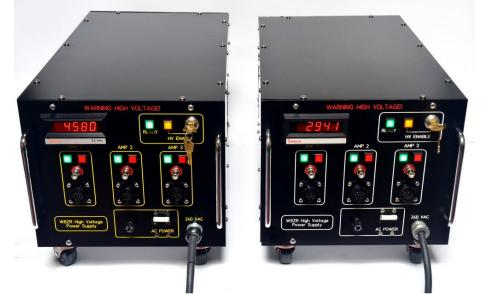
Figure 1: The high voltage power supplies, identical except for different voltage ranges, rest on the floor behind an operating table and independently power up to three legal-limit RF power amplifiers.
