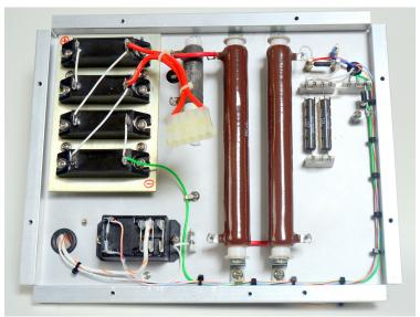
Figure 9: The bleeder resistors, metering components and HV– select relay mount on the rear of the subpanel. PTFE spacers insulate the bleeder resistors from the chassis, while the HV diode blocks are heatsinked to a 1/8 in. aluminum plate.
