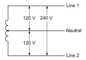
Also known as an Edison system, split-phase or centre-tapped neutral. This is the most common residential service in North America. Line 1 to neutral and Line 2 to neutral are used to power 120 volt lighting and plug loads. Line 1 to Line 2 is used to power 240 volt single phase loads such as a water heater, electric range, or air conditioner.
