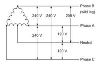
Also known as a high-leg or wild-leg delta system. Used in older manufacturing facilities with mostly three-phase motor loads and some 120 volt single-phase lighting and plug loads. Similar to the Three Phase Three Wire Delta discussed above but with a centre-tap on one of the transformer winding to create neutral for 120 volt single-phase loads. Motors are connected to phase A, B, and C, while single-phase loads are connected to either phase A or C and to neutral.
