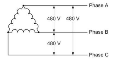
Used primarily in industrial facilities to provide power for three-phase motor loads, and in utility power distribution applications. Nominal service voltages of 240, 400, 480, 600, and higher are typical.
