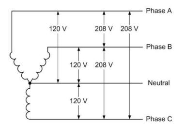
The most common commercial building electric service in North America is 120/208 volt wye, which is used to power 120 volt plug loads, lighting, and smaller HVAC systems. In larger facilities the voltage is 277/480 volt and used to power single phase 277 volt lighting and larger HVAC loads.
