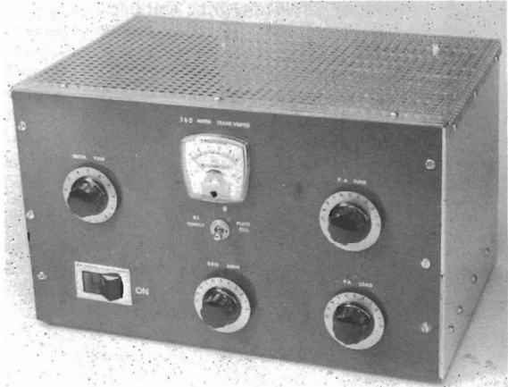
The transceiving converter is housed in a homemade aluminum cabinet which measures 8 × 8 × 12 inches. Perforated aluminum is used for the top and back sides of the cabinet to assure good ventilation.
