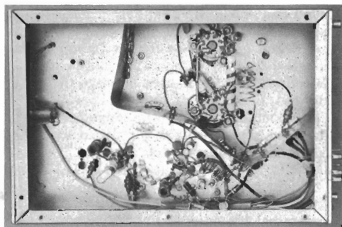
Bottom view—The oscillator, doubler, mixer and driver stages are below the copper partition which divides the chassis. The driver plate and amplifier grid coils are parallel to each other, just to the right of the amplifier tube sockets.
