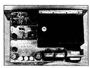
Top view of the BC-221 exciter designed to drive a crystal stage. The chassis is fitted around the BC-221 cabinet with the power supply at the rear and the additional r.f. amplifiers at the left.
