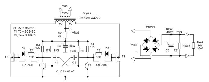
steering diode and 18k - much faster turn off, but again, nowhere near the mosfet's capabilities. The nett result is controlled switching edges, by using the gate - source capacitance as a low pass filter.
