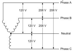
The most common commercial building electric service in North America is 120/208 volt wye, which is used to power 120 volt plug loads, lighting, and smaller HVAC systems. In larger facilities the voltage is 277/480 volt and used to power single phase 277 volt lighting and larger HVAC loads. In western Canada 347/600V is common.
