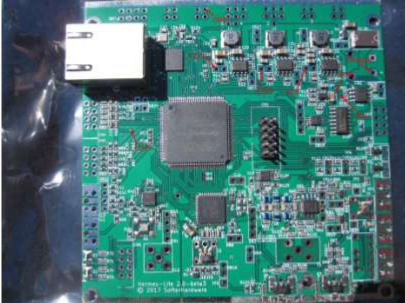
Hermes Lite 2, beta test PCB, awaiting fitting of through-hole components
