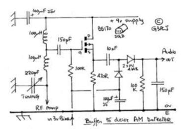
local TX) as well as covering the main frequencies of the Medium Wave band. The 3 volt bias for the extra BS170 buffer stage comes from the audio stages.
