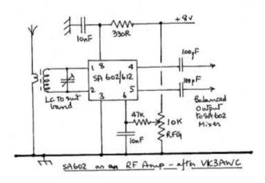
confident it works, and can also be used with single ended inputs and outputs if you wish - just RF decouple the unused input and ignore the unwanted output! G3PCJ
