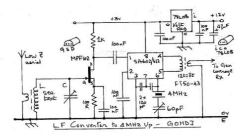
This scheme has the advantage that any of the LF bands can be used with a suitable RF filter on the front end! I have intentionally left the LC values off because I don't have them to hand but its not difficult to get something to resonate on any of those bands from 160m downwards; the low impedance aerial input winding should have about one fifteenth of the turns on the main resonant winding. The bands will translated from about 4.136 MHz up to nearly 6 MHz for 160m.
