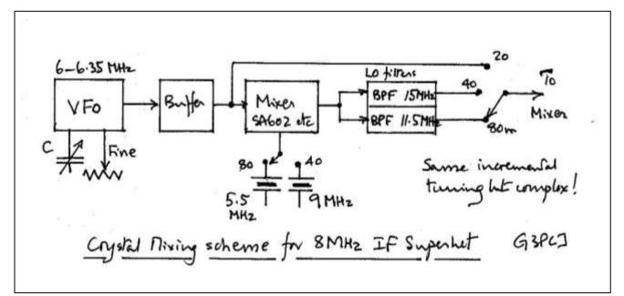
I think this could be improved for a three band rig doing 20, 40 and 80m by changing to a 9 MHz IF with a VFO at 5 - 5.5 MHz (in the classic 'image' scheme) for 20 and 80m. This needs to work on both sidebands but that is relatively easy! How do 40m? Use another complete VFO working 1.8 - 2 MHz! This is less complex than another set of filters and crystal mixing so is a good solution for the Somerton RX and Dorchester TX to replace the Minster & Lydford. G3PCJ
