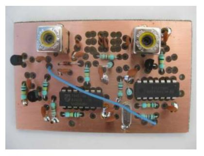
Although this type of mixer is not balanced for either input, it can perform well where the desired output is well removed in a frequency sense from the two inputs; this allows a double
