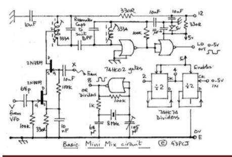
tuned filter (top of PCB) to be used for selection of either the sum or difference improve signal. То its versatility, the middle chip is a pair of digital dividers which can be arranged to divide either the crystal or the output by 2 or 4. This allows a 6 MHz VFO to be mixed with 8 MHz from a crystal to provide 14 MHz, then squared up & divided for 20, 40 and 80m. G3PCI
