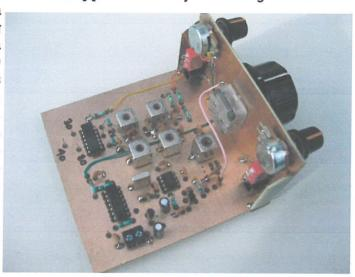
filters can use 3335 TOKOs and the VFO can use a TOKO 3333. As can be seen in the photo, it is not a complex PCB and the four individual (& simultaneous) outputs in top left corner, provide for easy band switching of any associated RX or TX!
