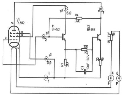
solid state equivalent on the right. For our purposes, ignore the "F" terminals and 56 ohm resistor; they were for television series heaters. The transistors can be MPSA 42's. T2 will need some heat sinking! Nowadays N channel power MOSFETs are cheap and can cruise with a kV on the drain. Replace T2 with a power MOSFET to suit your supply voltage [times two to be on the safe side]. Note that the suppressor grid [G3] is NOT implemented - no need.
