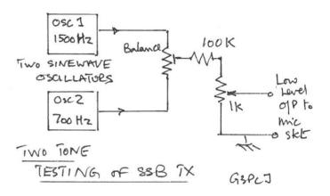
dio tone should be free of harmonics, otherwise the scope RF envelope will be a little fuzzy like that on the left below! The combined tones should have a level control so that it can replicate the low level output of your microphone.
