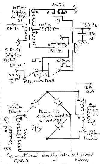
quite permissible to interchange the IF output point to the centre tap of the other RF transformer! Having made that step, the only remaining problem is to drive the LO transformer!
