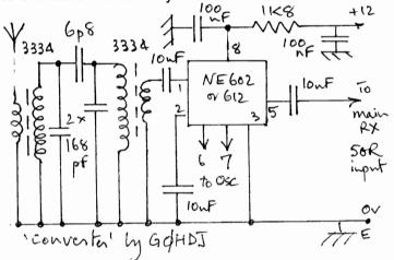
receiver. This is a potential divider giving attenuation of about 30 times - this is the main reason why the converter was so deaf! A buffer or impedance converting transformer is needed.
