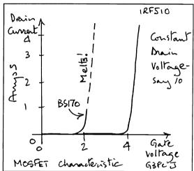
current. The device is also highly suitable as a buffering source follower with unity voltage gain. Since the device bandwidth is very large (well into VHF) there is the potential for unintended oscillation unless a 'gate stopper resistor' is added – this need be only a few Ohms but can be higher depending on the desired actual bandwidth.
