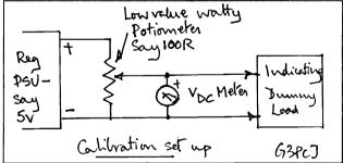
dBm figures are the RMS power (being dissipated) relative to 1 mW (0 dBm) into 50 Ohms. The higher ranges each increase power by a factor of 10 which corresponds to a 10 dB increase giving FSDs of 27 & 37 dBm or 0.5 & 5 Watts. The maths behind the calibration is  $V_{DC} = \text{sq.root(2RP)}$ , where P = 50 Ohms & P = power in watts.
