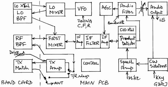
The main PCB is  $100 \times 160$  mm with the band cards ( $50 \times 160$  mm) being inserted vertically along the rear edge. The card switch PCB has to be mounted immediately behind the main PCB. Both it and the counter PCB are  $160 \times 50$  mm. In addition a meter kit is available to provide an S meter (with extra audio derived AGC) and a resistive transmitter matching bridge plus output indicator.
