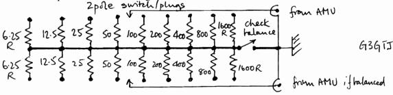
Checking balance is very simple. Load the balanced output of the AMU with a load of two equal resistors in series (balance switch open). Adjust the AMU for 1:1 SWR at the AMU input and then connect the mid point to ground by closing the balance switch. Any change in SWR will indicate unbalance within the AMU. Baluns can also be checked this way and their losses established using the AMU test procedure.
