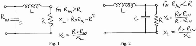
The formulae for calculating the values of inductance and capacitance assume that "R" is a pure resistance. In practice it is more than likely that there will be some reactance associated with it which will modify the values of inductance and capacitance required. This is accommodated for by making them variable, using a variable capacitor and either a tapped coil or a "roller coaster" for the inductance. These arrangements are shown in Figs. 3 and 4.
