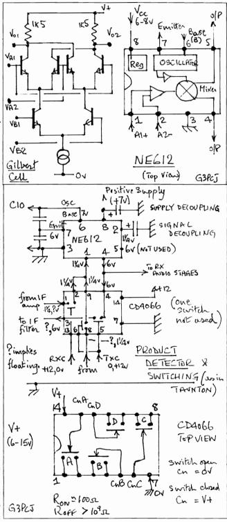
seldom over a volt p-p ontop of the DC voltage of about 1.25 at the input or about 5 to 6 volts DC at the outputs. To help explain the switch connections in the 4066 I have drawn out its pin connections separately. Each switch in a 4066 has a resistance of about 100 Ohms when **on** suggesting that it should only be used where the circuit impedances are significantly above this figure - hence its use with the 1K5 in and out
